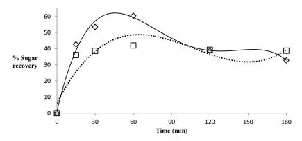
FIG. 4. Achieved percent of sugar recovery of released of mango skin during dilute acid hydrolysis with 2% by weight of acid subjected to different pretreatments ( $\Diamond$  = immersion in water for 24 h and  $\Box$  = autoclaved water for 1 h).
