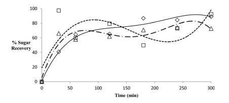
FIG. 3. Percent sugar recovery of mango skin with dilute acid hydrolysis at different times and concentration of acid ( $\Diamond = 1\%$  w/w,  $\Box = 2\%$  w/w, and  $\Delta = 5\%$  w/w).
