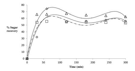
FIG. 6. Percent sugar recovery of pine wood with dilute acid hydrolysis at different times and concentration of acid ( $\Diamond = 1\%$  w/w,  $\Box = 2\%$  w/w, and  $\Delta = 5\%$  w/w).
