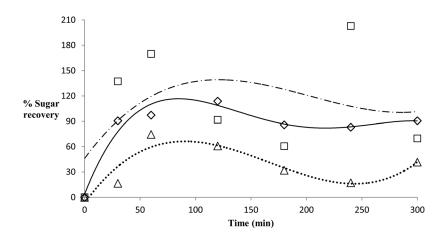
FIG. 5. Percent sugar recovery of mango bagasse with dilute acid hydrolysis at different times and concentration of acid ( $\Diamond = 1\%$  w/w,  $\Box = 2\%$  w/w, and  $\Delta = 5\%$  w/w).
