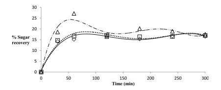
FIG. 1. Percent sugar recovery of sugarcane bagasse with dilute acid hydrolysis at different times and concentration of acid ( $\Diamond = 1\%$  w/w,  $\Box = 2\%$  w/w and  $\Delta = 5\%$  w/w).
