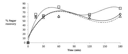
FIG. 7. Achieved percent of sugar recovery of pine wood during dilute acid hydrolysis with 1% by weight of acid subjected to different pretreatments ( $\diamond =$  immersion in water for 24 h,  $\Box =$  autoclaved water for 1 h,  $\Delta =$  autoclaved 1% NaOH for 1 h, and  $\times =$  alkaline hydrolysis).
